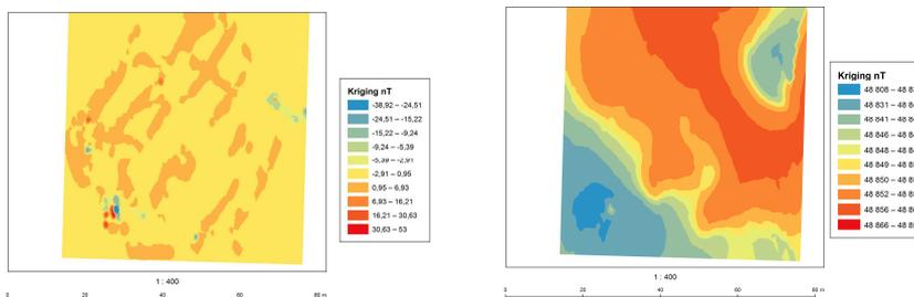
**Fig. 4: Magnetometric data interpolation using kriging method for magnetic field intensity (left) and for gradient of magnetic field intensity**
