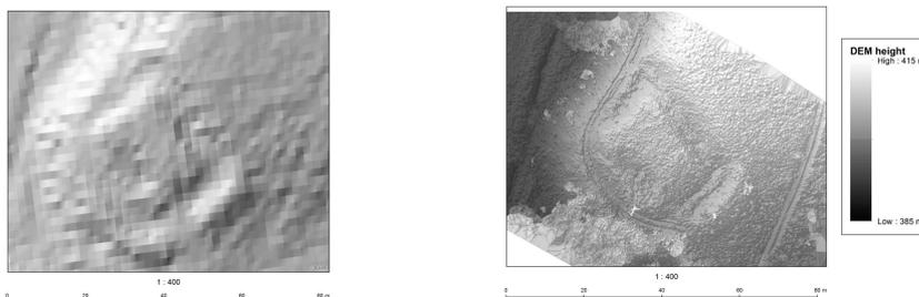
**Fig. 2: Hill Shaded Terrain Model: COSMC – image service (left) and derived from RPAS**
